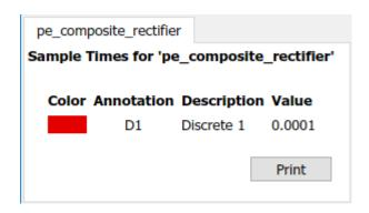
The model is running at a discrete rate, therefore it is using a fixed-step solver, with a sample time of 1e-4 s.
